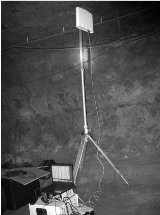
Fig. 5. Tx unit for WiMax 1,5GHz system
