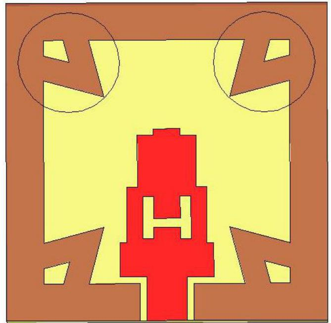
Fig. 7. Geometry of the antenna with four semi-triangles metallic strip in comparison of proposed antenna with two circular grounded strip.
