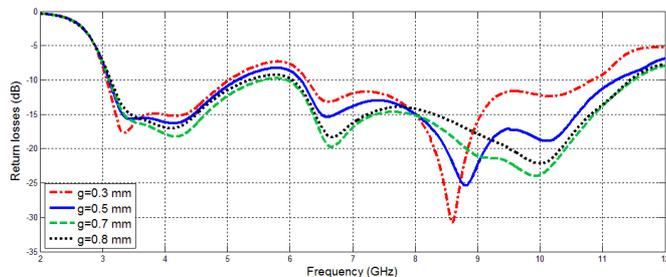
Fig. 6. Simulated reflection coefficients of the proposed antenna with different value of gap distance ( $g$ ) with a fixed values of  $P_1=4.4$ ,  $P_2=4.5$ ,  $L_s=18.8$  and  $T_2=4.8$  (Units are in mm).
