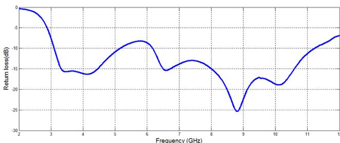
Fig. 2. Simulated reflection coefficient of the proposed antenna.
