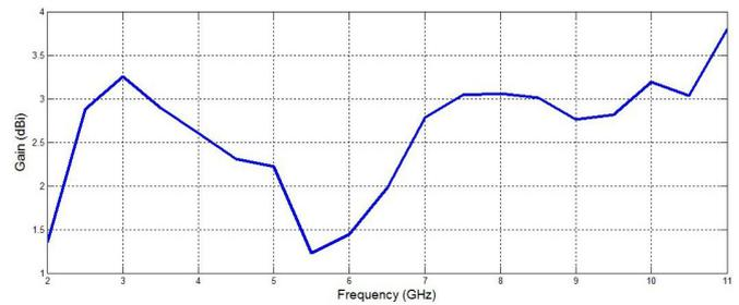
Fig. 11. Measured gain of CPW-fed monopole antenna.
