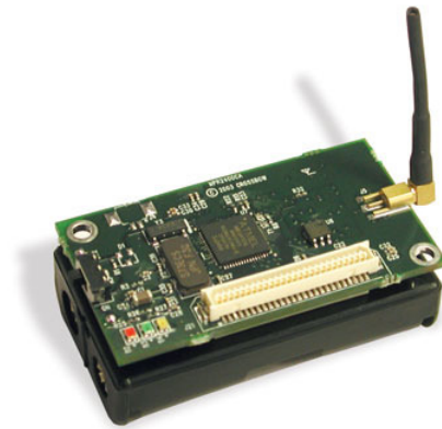
Fig. 1. MICAz mote for which the idea is proposed. These motes lose their battery voltage with the passage of time.
