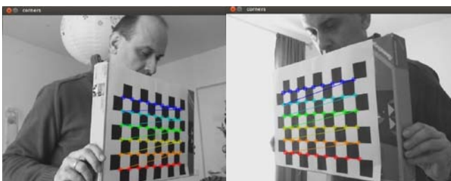
Fig. 7. Checkboard pattern stereo vision
