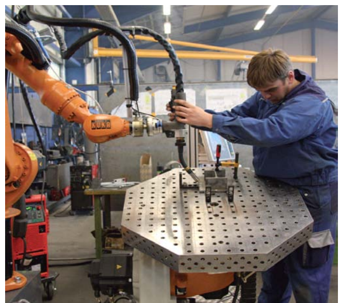
Fig. 1. Programming by demonstration [2]
