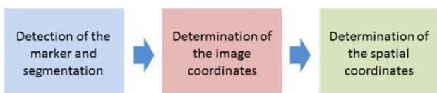
Fig. 3. Image processing process chain
