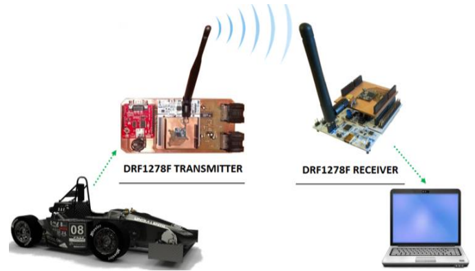
Fig. 4. Base station on the right with DRF1278F radio module in reception mode connected with PC through a ST Nucleo board and realized telemetry system on the left inside the car for data sensors detection and transmission.
