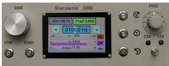
Fig. 6. User interface (front panel of the controller)
