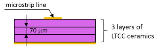
Fig. 5. Cross-section of the designed multilayered microstrip
