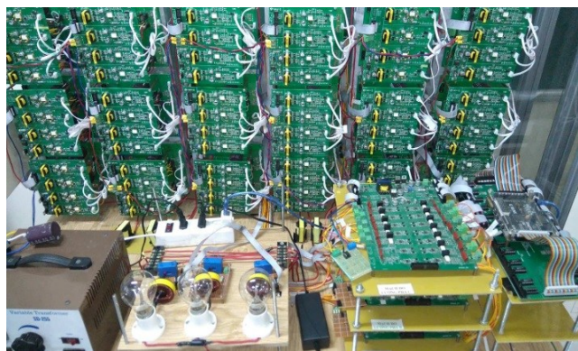
Fig. 8. Experimental system of MMC: 1. Driver; 2. V_{DC} ; 3. Load; 4. Measure circuit; 5. FPGA; 6. ADC
