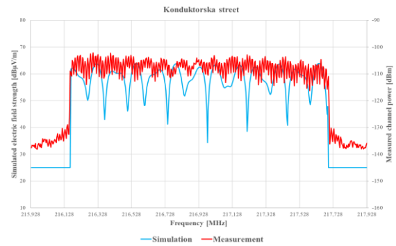
Fig. 10. Comparison of simulated (simulation based on channel power measurements) and measured fades on Konduktorska street. Simulated fades depth up to 27 dB, measured fades depth up to 10 dB.
