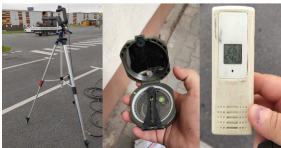
Fig. 4. Tripod with directional antenna, compass, temperature and humidity meter [22]
