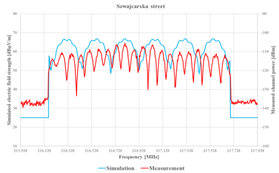
Fig. 15. Comparison of simulated (simulation based on channel power measurements) and measured fades on Szwajcarska street. Simulated fades depth up to 17 dB, measured fades depth up to 25 dB
