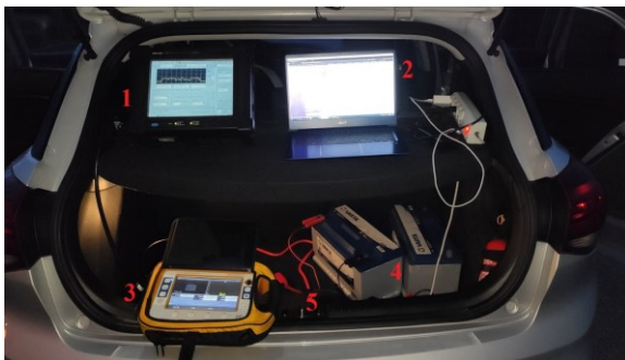
Fig. 5. Equipment of the measuring station (1 - spectrum analyzer, 2 - computer, 3 - Promax HD Ranger +, 4 - batteries, 5 - converter) [22]
