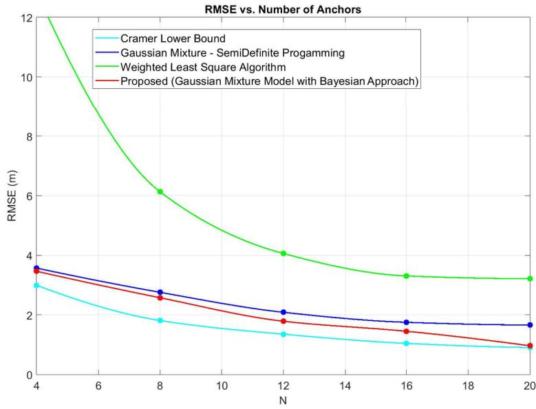
Fig. 3. RMSE versus the number of anchor nodes
