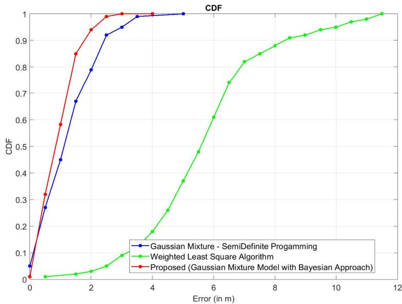
Fig. 4. CDF of localization errors for the different algorithms
