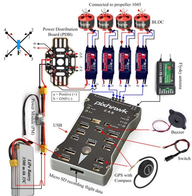
Fig. 2. The DIY of quadcopter using Pixhawk 2.4.8 and their basic connection for our work.
