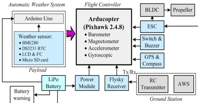
Fig. 5. The designed of quadcopter for implementing PBL in Atmospheric Physics.
