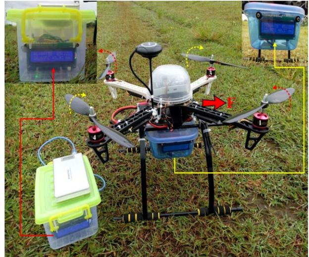
Fig. 6. A quadcopter that has been developed and is equipped with Arduino meteorological sensors as payload (light blue box) and AWS for ground-station (yellow box).
