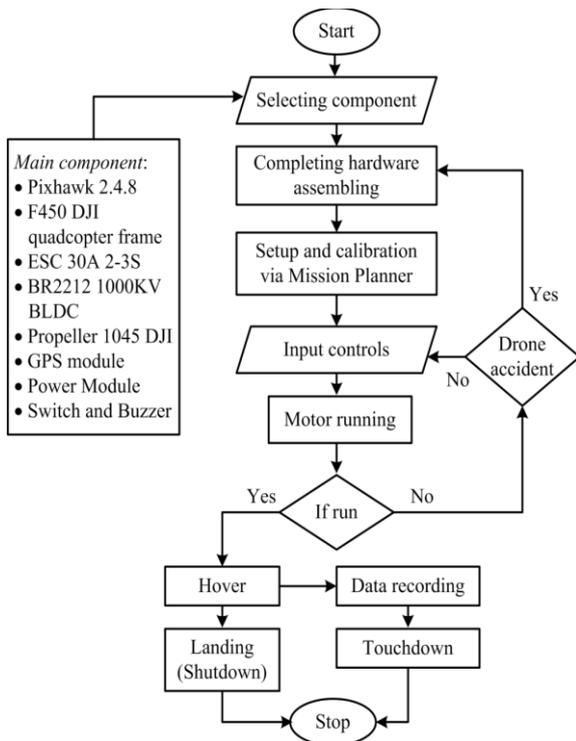
Fig. 1. The flow of how the quadcopter control system works in this study.
