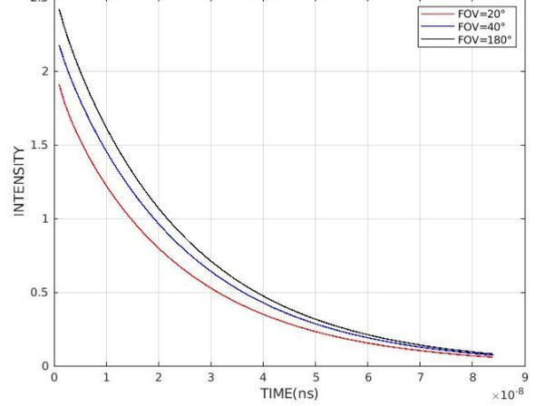
Fig.4. Impulse response of the channel with L=45.45 m of coastal water
