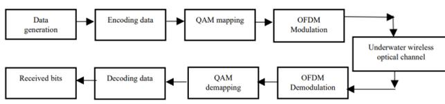
Fig. 1. Block diagram of QAM-OFDM mapped underwater wireless optical communication
