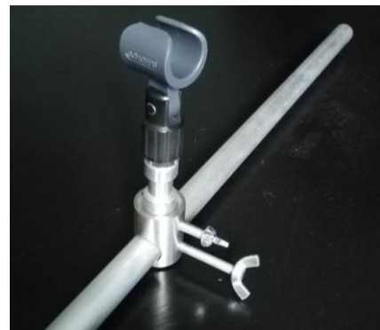
Fig. 6. Microphone holder positioned on the aluminum section
