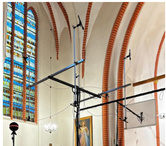
Fig. 4. 3D microphone array build by the authors for the purpose of immersive recording session
