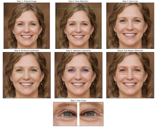
Fig. 4. Step-by-step visualization of the preprocessing pipeline, including landmark extraction and eye image cropping.
