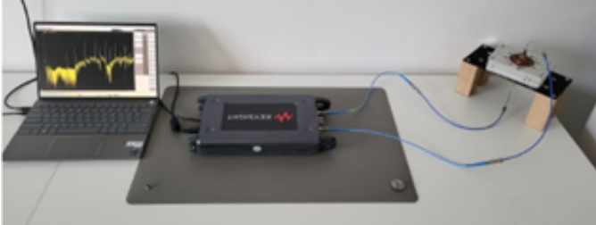
Fig. 2. Q-SSR whole measurement setup with sample inserted into air slot.
