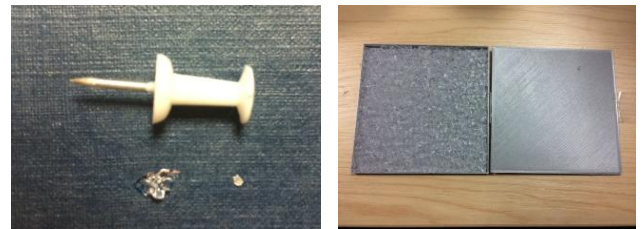
Fig.7. A comparison between one crystal of the Polyacrylamide gel with a one that absorbed water and how the water absorbed gel lay out in the 3D box with its cover underneath the used antenna
