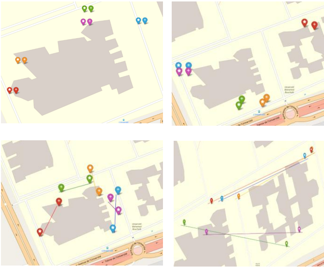
Fig. 5. Some examples of ground-truth locations and RF predicted positions. (a) excellent positioning (b) good positioning (c) moderate positioning (d) poor positioning
