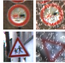
Fig. 2: Examples of the generalized data augmentation (right) applied to GTSRB traffic sign images (left). Each sample was simultaneously subjected to four distinct environmental distortions : random rotation, simulated rain, Gaussian blur, and brightness level shifts.
