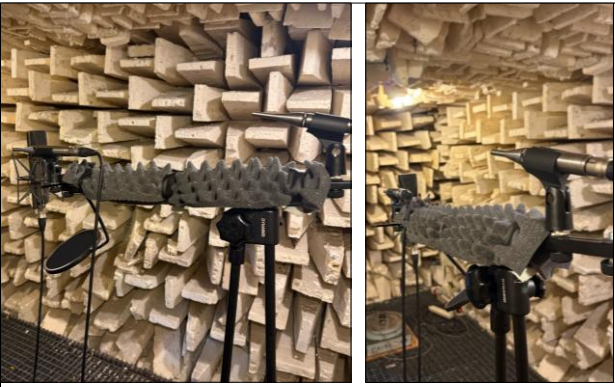
Fig. 4. Microphone arrangement using a single stand with damping foam on the beam (System A)
