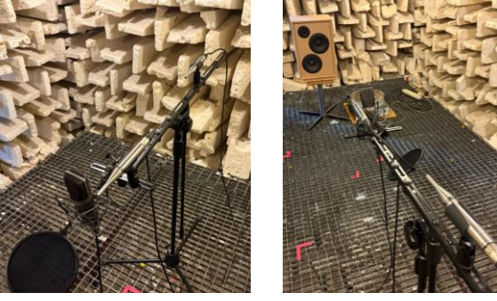
Fig. 3. Microphone arrangement using a single stand without damping foam on the beam (System A)
