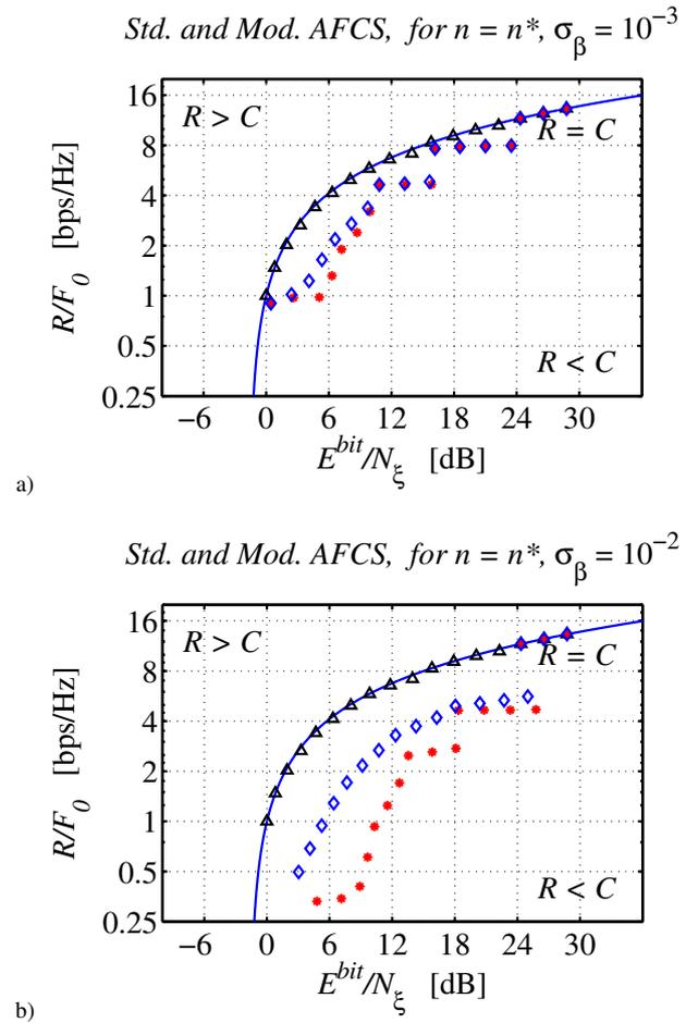
Fig. 10. Experimental power-bandwidth efficiency for standard (red stars) and modified (blue diamonds) AFCS, for  $\sigma_\beta = 10^{-3}$  V (a),  $\sigma_\beta = 10^{-2}$  V (b), and for SNR changing from 0 to 40 dB (from bottom to top).
