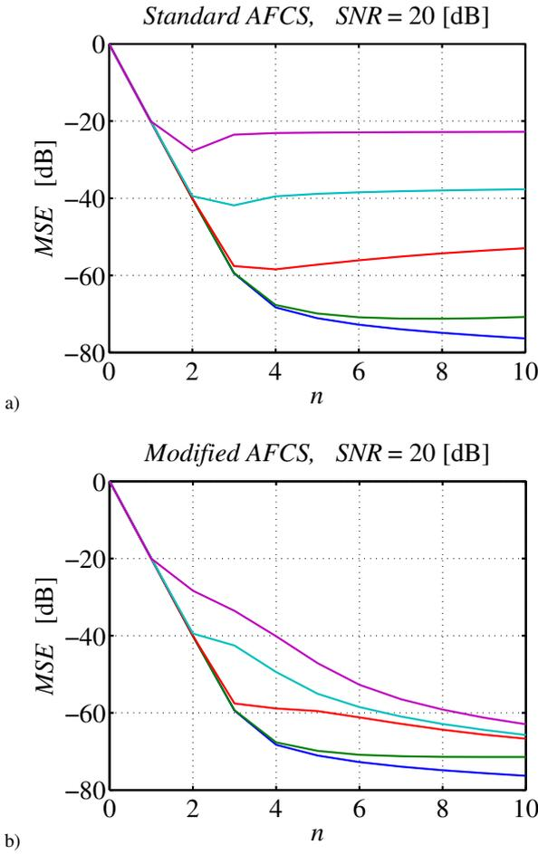
Fig. 5. MSE for standard (a) and modified (b) AFCS, for different values of drift rate  $\sigma_\beta = 10^{-6}, 10^{-5}, 10^{-4}, 10^{-3}, 10^{-2}$  V (lines from bottom to top, respectively) under SNR = 20 dB.
