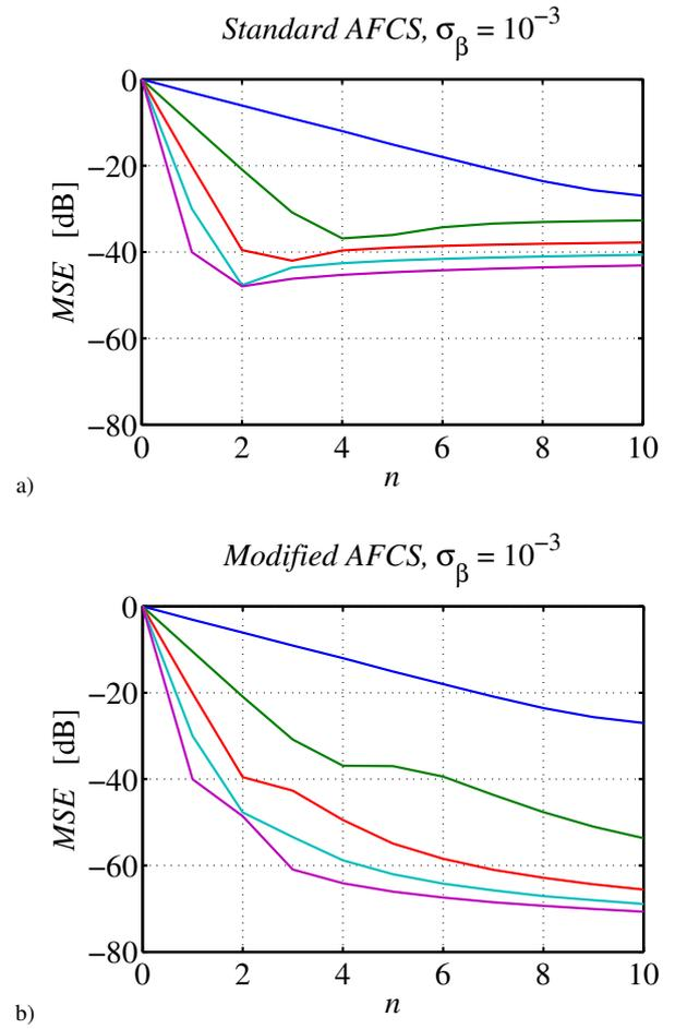
Fig. 6. MSE for standard (a) and modified (b) AFCS, for different values of SNR = 0, 10, 20, 30, 40 dB (lines from top to bottom, respectively) and standard deviation of drift rate  $\sigma_\beta = 10^{-3}$  V.
