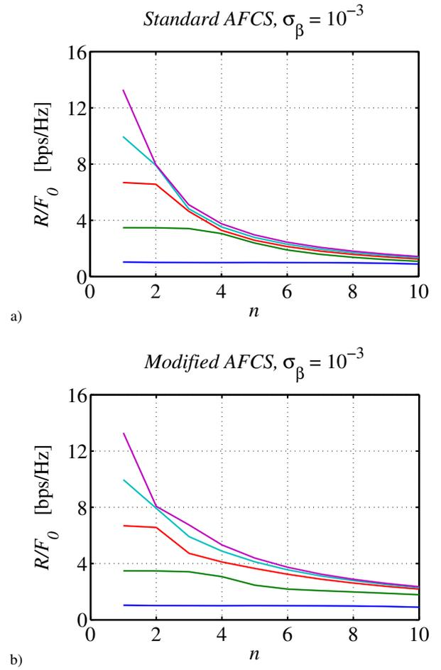
Fig. 8. Transmission bit-rates for standard (a) and modified (b) AFCS, for different values of SNR = 0, 10, 20, 30, 40 dB (lines from bottom to top, respectively) and  $\sigma_\beta = 10^{-3}$  V.
