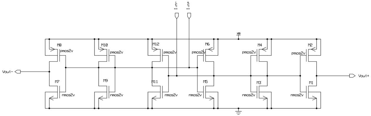
Fig. 3. Schmitt trigger used in the comparator.
