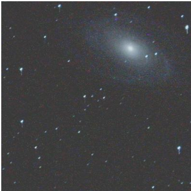
Fig. 9. Picture of the M81 Galaxy taken with drive inconsistent with sky revolution. Refractor SW 80ED, 80mm/600mm, Canon 300D, ISO 800, one exposure 300 s. Photo: Robert Suszynski.
