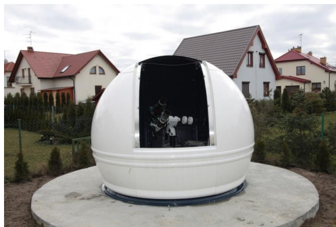
Fig. 1. A stand-alone, remotely controlled station for DSO astrophotography.
